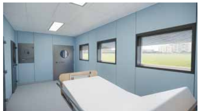
Patient room with door to patient entrance sluice material transfer box for sample transfer to BSL-3 laboratory
