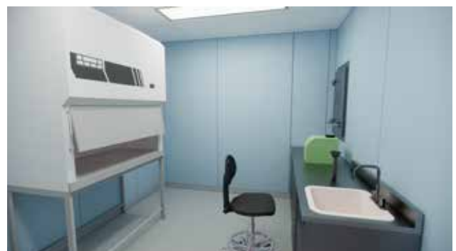
BSL-3 laboratory with Biosafety Cabinet (BSC)
